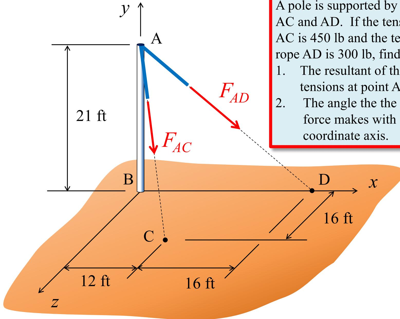
A pole is supported by two cables; AC and AD. If the tension in rope AC is 450 lb and the tension in rope AD is 300 lb, find:
